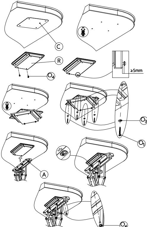
**NOTE:** If mounting to a wood beam ceiling, ensure the front and back holes are used for the main support if mount is in line with the beam. If perpendicular to the beam, use keyhole openings for the main support. **Do NOT** use included Concrete Anchors (O2) for wood or drywall.
