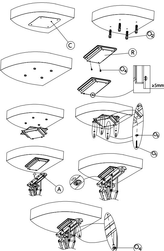
**⚠ NOTE: O1 Concentric installation, do not tilt installation**
